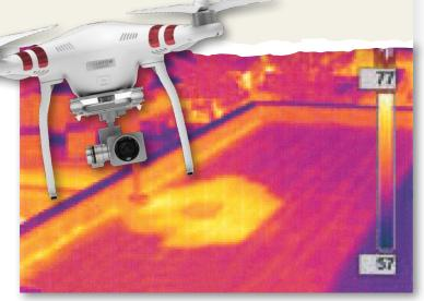
This drone photo using our infrared scan clearly shows the penetration of moisture which is represented in the color changes across the roof from dark to glowing red.
